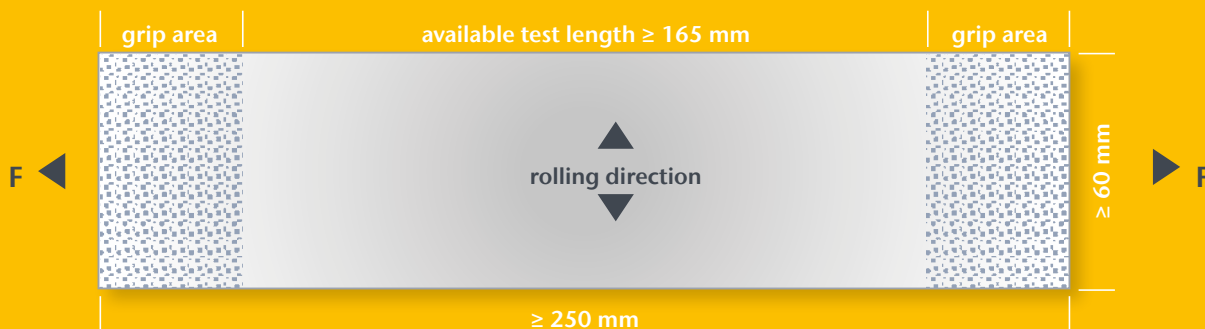
1 Sample dimensions, location of the sample to rolling direction and direction of pre-strain
