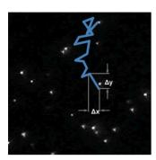
Nanoparticle Tracking Analysis (NTA) is a widely used technique to characterize nanoparticles in liquids. It combines laser light scattering and video microscopy to visualize and track the Brownian motion of individual particles. By analyzing their movement, the particle size (hydrodynamic diameter) and concentration can be determined using the Stokes-Einstein equation.
