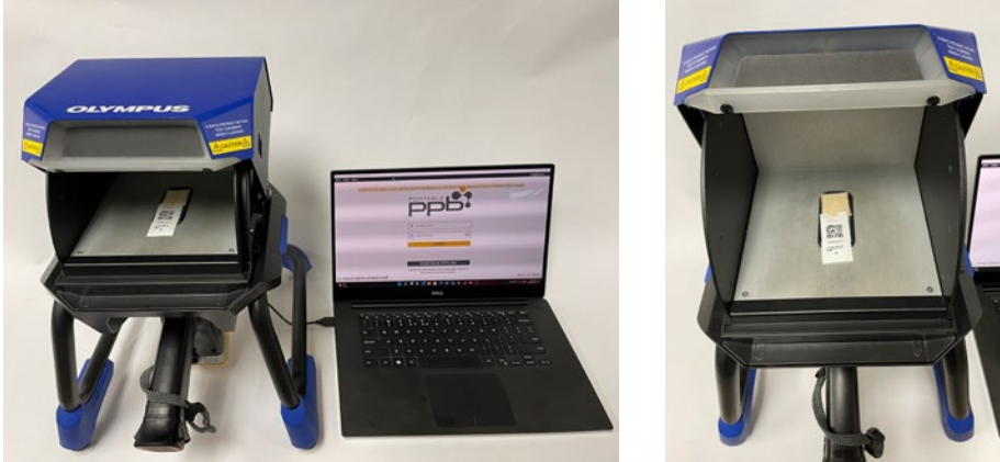
Figure 1: Analysis of a detectORE™ collector device in a Vanta Work Station using PPPB pLIMS software.
