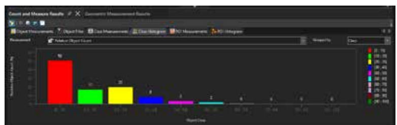
Histogram displaying relative object count (%) per particle size class
