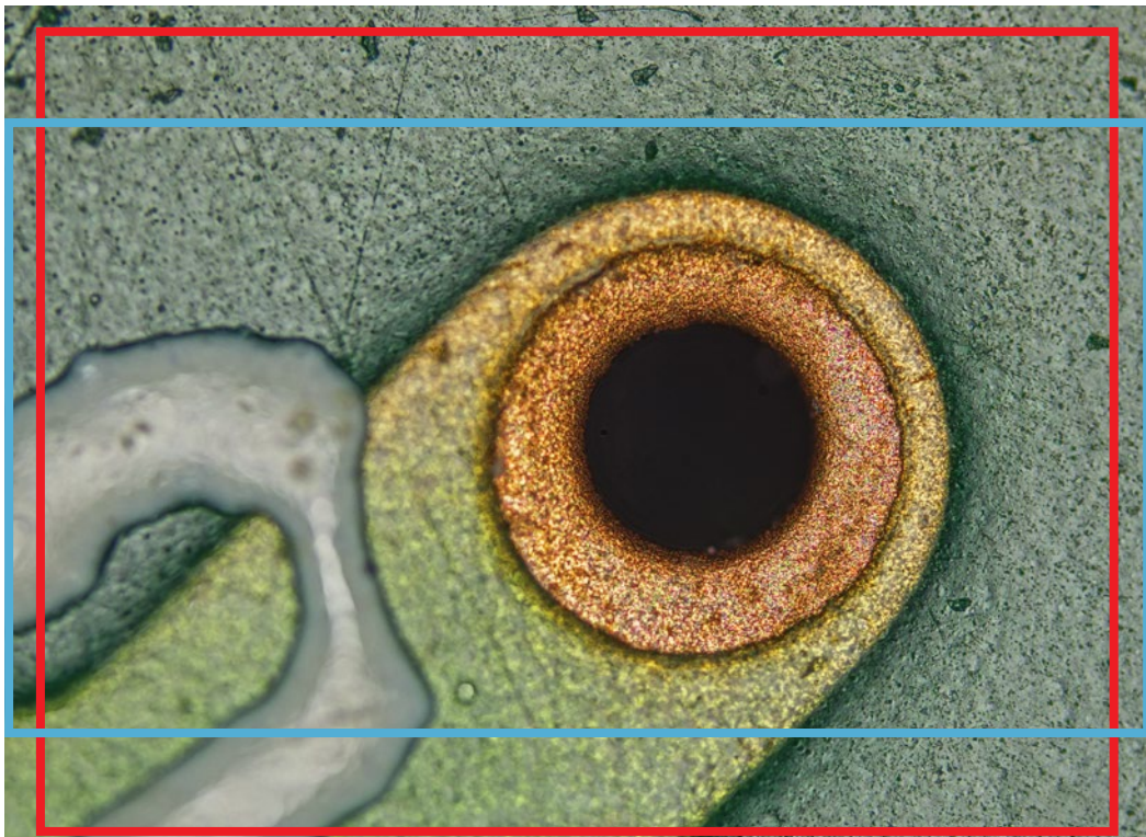
The DP75 camera's field of view when used with the 0.63× camera adapter (red frame) compared to the DP74 (predecessor) camera's field of view when used with the 0.63× camera adapter (blue frame)
