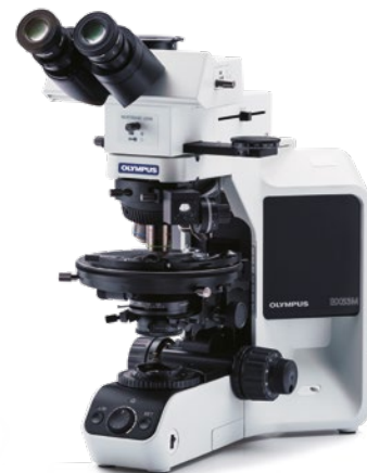
BX53M conoscopic/ orthoscopic configuration
