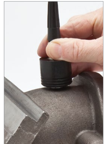
Many cast metal parts or highly attenuating materials can be measured with the High Penetration software option.
