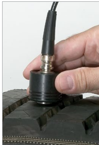
Measure depth to steel ply / cords in rubber conveyor belts or tires.
